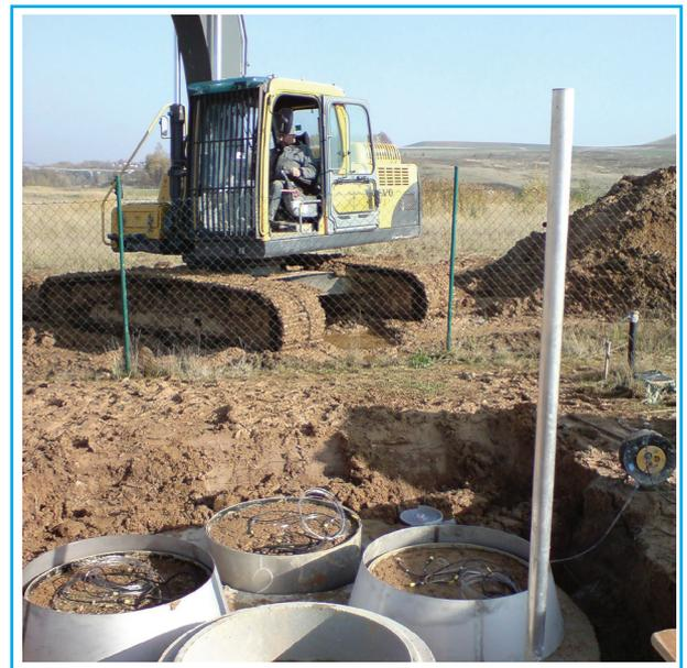
2008: 3-Channel Lysimeter station Friedrich-Schiller-Universität Jena: 1 x monolithic extracted lysimeter, 2 x filled lysimeters, gravity lysimeter.
