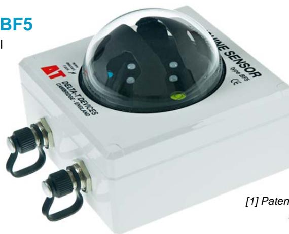
The BF5 uses this information to calculate whether the sun is shining and to measure the direct and diffuse components of solar radiation, avoiding the need for the shade ring adjustments required with conventional diffuse light sensors (levelling is the only adjustment required).
