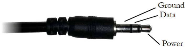
Figure 8: 3.5 mm Stereo Plug Wiring
