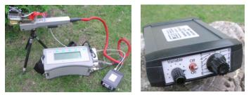
The PLU5 can be used to maintain a single constant light concentration within the leaf chamber or be used to generate data for rudimental A/Q (light response) curves.
