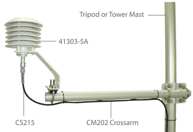
To attach the 41303-5A to a CM202, CM202SS, CM204, CM204SS, or CM206 crossarm, place the 41303-5A's U bolt in the bottom holes.
