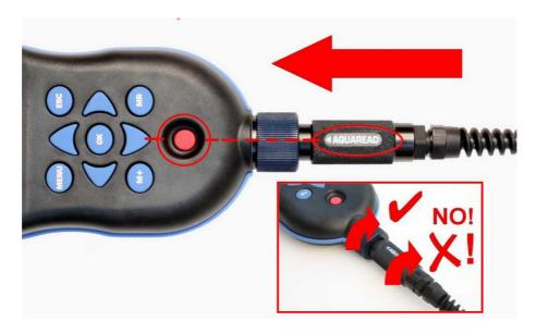
Always ensure the Aquameter<sup>®</sup> is switched off prior to connecting or disconnecting an Aquaprobe<sup>®</sup>. Align the **◄Aquaread**<sup>®</sup> logo on the plug body with the red on/off switch on the Aquameter<sup>®</sup>, then press the plug into the socket and tighten the retaining collar.
