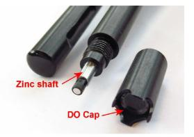
**NEVER re-install a Galvanic DO Membrane Cap once it has been fully tightened.** The membrane will be stretched and will not seal properly over the silver cathode a second time. If the membrane does not create a proper seal over the silver cathode, the DO sensor will not operate correctly and any readings given will be erroneous.
