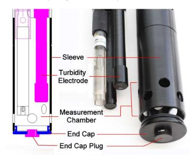
In order to obtain consistent results, the measurement chamber created within the Aquaprobe® must remain physically constant during both calibration and measurement.
