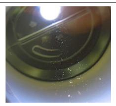
This level of aeration will register the equivalent of around 5NTU as each bubble is seen as a solid particle.
