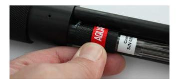
Slide the lanyard over the electrode and use it to grip the knurled body.
